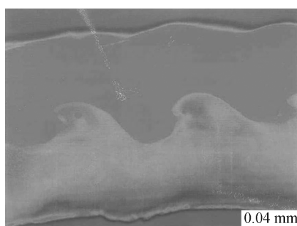
Fig. 11 Photograph of extrudate cross-section wave interlocking
